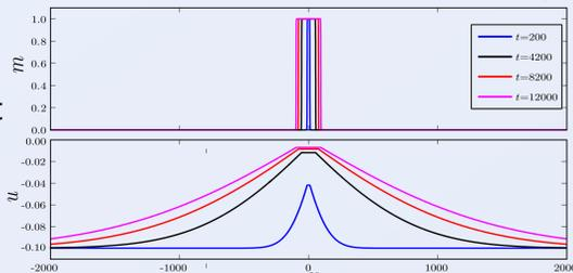
Order parameter and temperature profiles for  $p=5 \cdot 10^{-3}$ , low undercooling. Order parameter interface width  $2^{1/2}$  in dimensional units. Thermal profile much wider.
