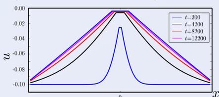
Temperature profile for a system with nearby boundaries kept at the undercooling temperature. Note the difference before and after the field widened to the system size.
