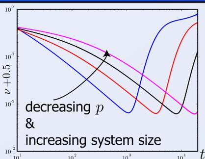
Growth exponent for increasing  $p$  and increasing system size. When temperature profile width exceeds the system size, the exponent grows.
