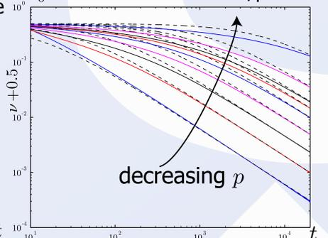
Growth exponent  $\nu + 0.5$  versus time for (exponentially) decreasing  $p$ . Dotted lines are fitted to  $1/2(1 + t_0/t)^{-1}$
